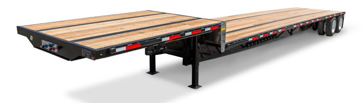
Our rugged steel drop deck trailer is built to last. Heattreated 130ksi steel provides high strength and low trailer weight. In addition, the premium paint process ensures best-in-class corrosion resistance and keeps your trailer looking good year after year.
